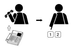
**Step 2.** Following a brief call tone, the master station is automatically connected to the substation. The master station's voice is heard at the substation while the master station operator is talking, and the substation's voice is only heard at the master station when the master station operator stops talking.
